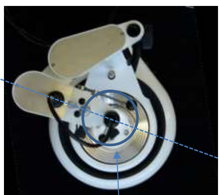
Radius of movement of the milling spindle after rotation of the milling shell for processing telescope No.2
